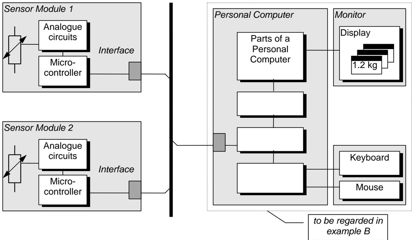
**Figure 6-2:** Example B: PC-based, Modular Complex Measuring System
