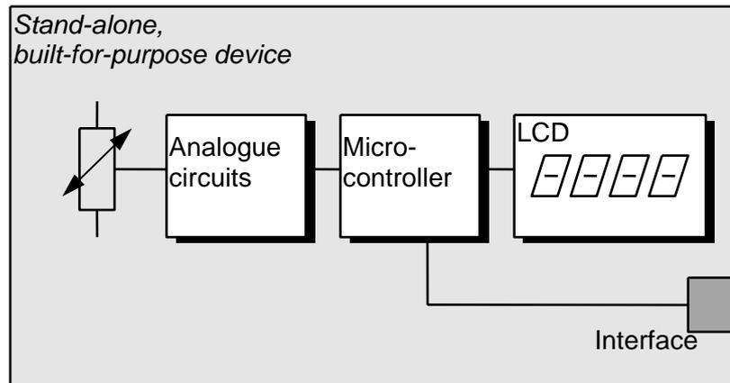
**Figure 6-1:** Example A - Simple Stand-Alone Measuring Instrument
